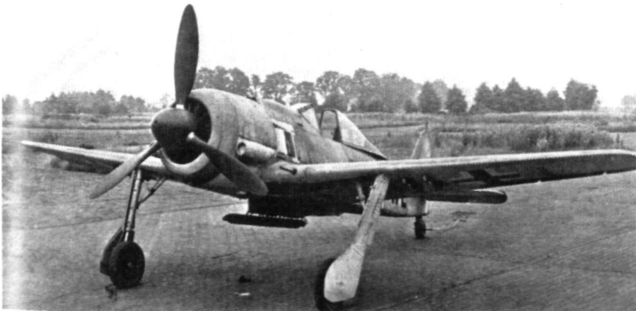
The Focke-Wulf FW 190 started to replace the Ju 87 in 1943. It was less accurate but far more survivable owing to its greater speed, and two dedicated attack variants were produced. This FW 190F-8 has a dust filter on the port side of the engine. (Bruce Robertson)
