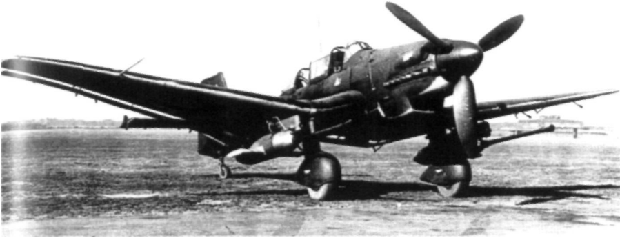
The Junkers Ju 87G was essentially the D model fitted with a 37mm cannon pod under each wing, which ruled out a steep diving attack. As a tank-buster it was lethal in the hands of an expert, but the pods adversely affected handling, and it was no aircraft for a beginner. (Bruce Robertson)
