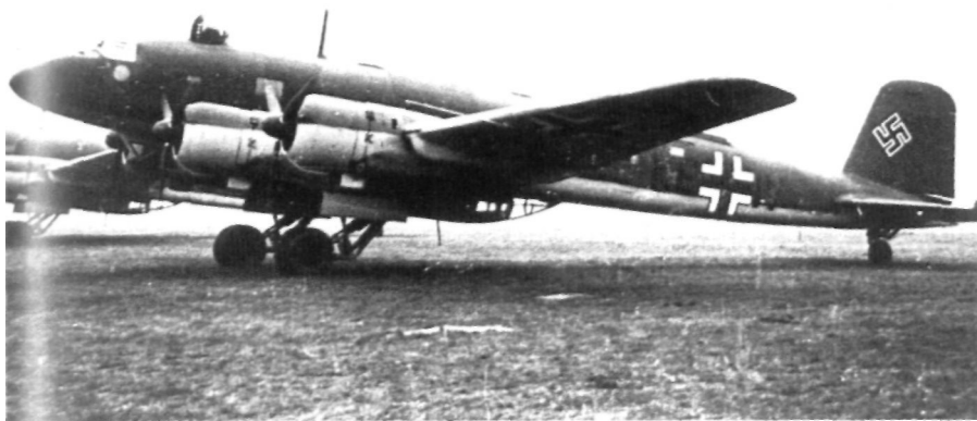
The Focke-Wulf FW 200C caused untold damage to Allied shipping in the Atlantic, but there were never enough of them to be really effective. Moreover, it was not really strong enough to withstand the stresses and strains of operations. (Bruce Robertson)
