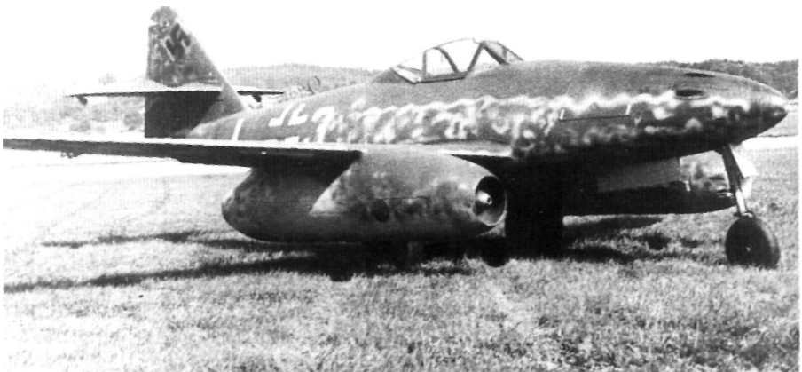
The Messerschmitt Me 262A was adapted as a fighter-bomber to become the Sturm-vogel, but speed and manoeuvrability were degraded by external loads, while bombing accuracy was hard to obtain, even in shallow diving attacks at low level. (Bruce Robertson)
