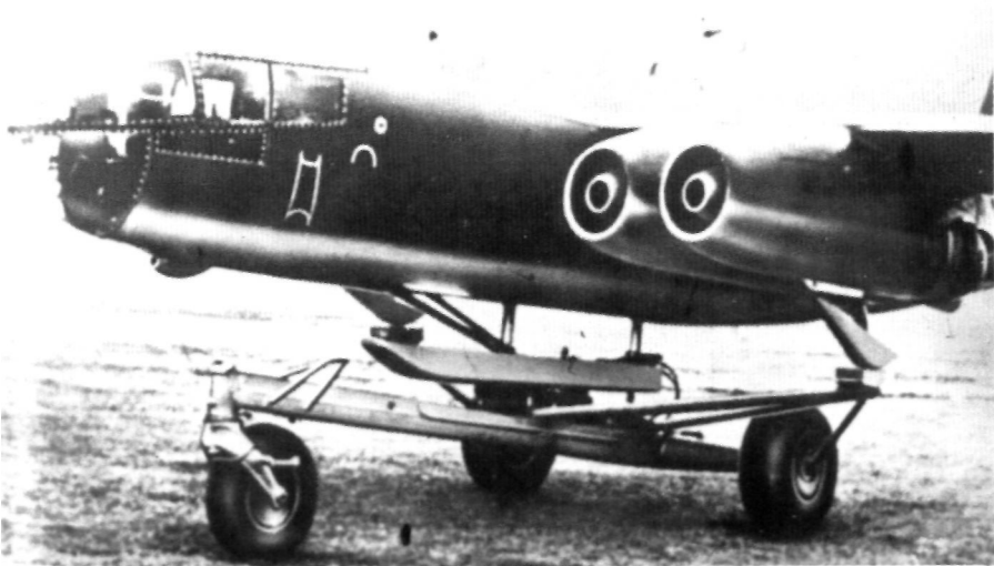
The Arado Ar 234 was the world's first operational jet bomber. It was normally twin-engined, but this experimental four-engined variant reveals in detail the launching trolley and triple skid undercarriage featured on all early aircraft.
