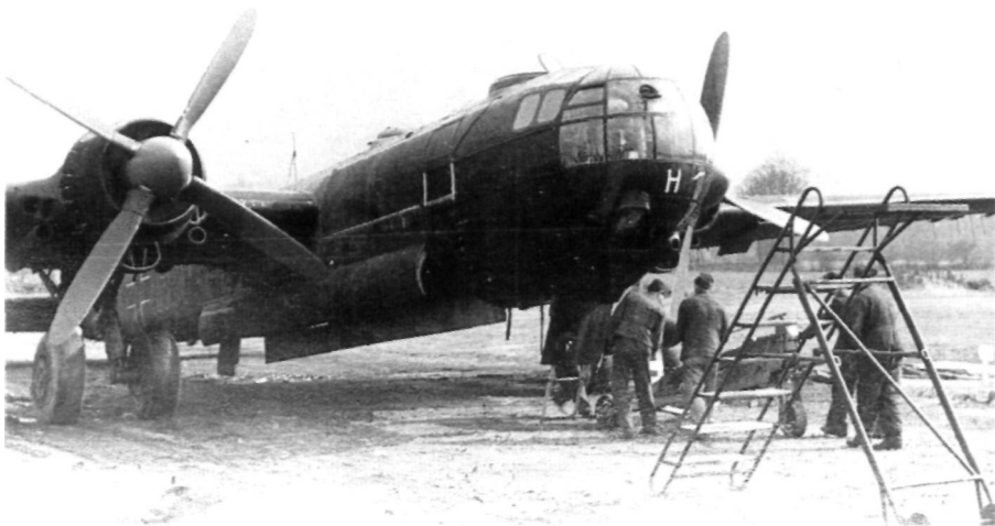
With coupled engines driving two huge four-bladed propellers, the Heinkel He 177A was the nearest the Luftwaffe ever got to having a true strategic bomber. It was endlessly delayed by engine fires caused by the unconventional layout, and by the time the problems were solved it was too late. (Bruce Robertson)
