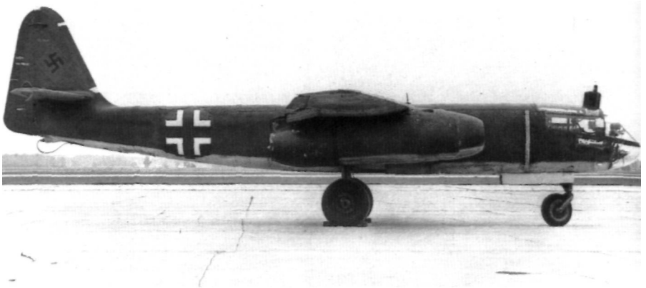
The trolley and skid arrangement proved too unwieldy for operational use, and the final variant of the Ar 234 had a conventional tricycle undercarriage. The projection above the cabin is a periscopic bomb sight for use in shallow diving attacks. (Bruce Robertson)
